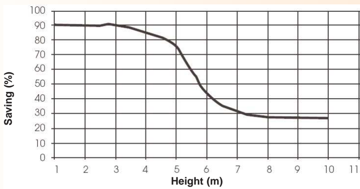
Normal energy saving with hot-air curtain
